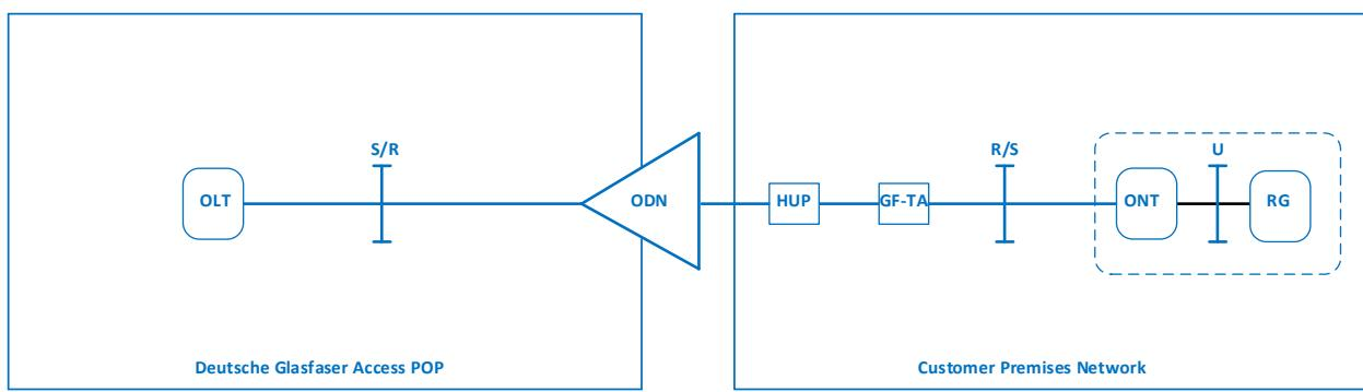
IF<sub>PON</sub> denotes the interface at reference points S/R and R/S. This interface must support all protocols that are necessary for transmission between OLT and GPON and XGS-PON ONT's/ONU's.
